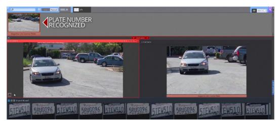
**Configure automatic scenarios when a match is found.** For instance, notify the operator when the recognized number is on the negative watchlist or open the barrier when the number is on the access list. ANPR runs on the server side or on supported LPR/ANPR cameras.
