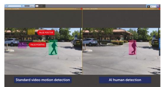
When applied to the **Object Tracker**, the neural network accurately detects specific types of moving objects, e.g. humans or vehicles. This technology can filter out false alarms in busy scenes where multiple moving objects might interfere with the results. You can apply any conventional video analytics (loitering, line crossing, object appearance and disappearance, etc.) to the detected objects.
