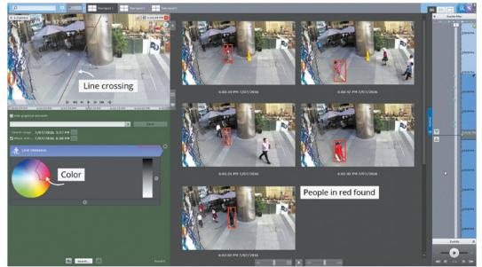
**MomentQuest analyzes live video** and generates a stream of metadata — a lean description of moving objects within the scene — which is recorded along with video stream. To retrieve recorded footage of an event of interest, just enter specific criteria: motion in area(s), crossing of a line, object color or size, etc. Within seconds the system displays thumbnails of relevant video episodes. Save a search query for later use on any camera.
