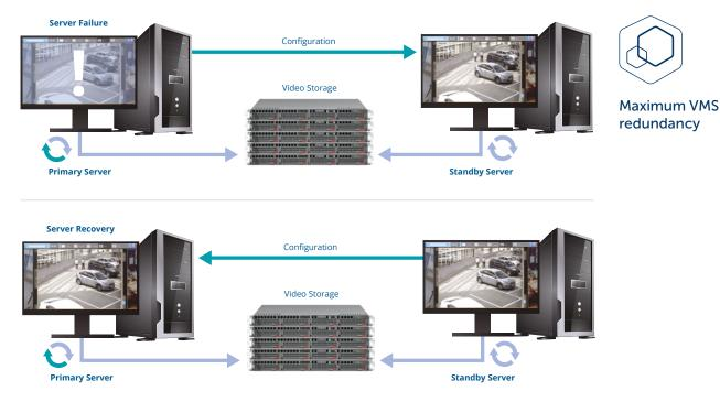
**Failover quickly switches** to a standby server when communication with the primary server is lost. The standby server automatically takes over all functions from the offline or malfunctioning server. Live video streaming and recording resume immediately. You can suspend any server in the cluster with no system downtime, e.g. for maintenance.
